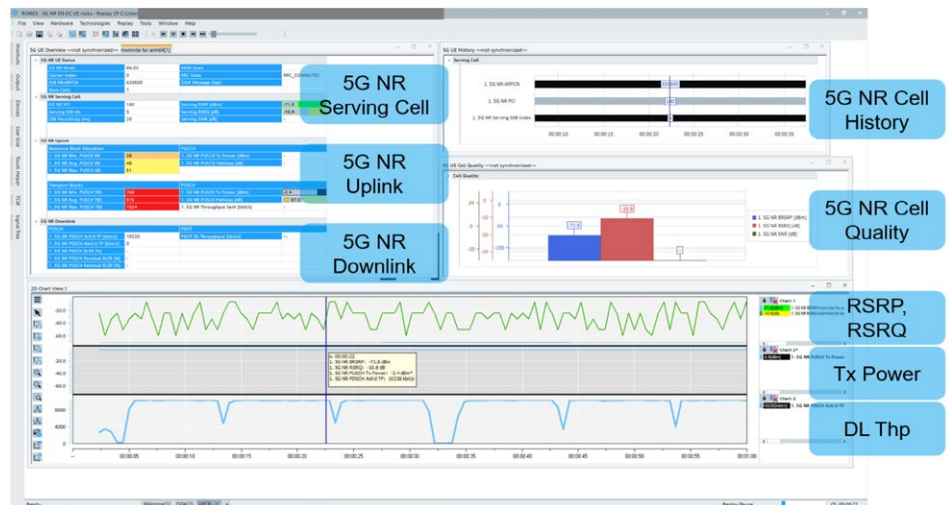
Figure 9: 5G user equipment measurements with the R&S ROMES4 software suite – Source: Rohde & Schwarz.
